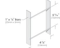
Light and airy, the Opus70 design provides for a modular perimeter fence that blends into the background while providing a permanent physical barrier. Extra wide spacing reduces visual impact, but does not meet IBC infill requirements with regards to opening size.
