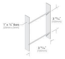
The timeless square pattern of Opus60 complies with IBC spacing requirements for infill panels of all types. The open matrix minimizes visual obstruction to attractively maintain security and code compliance.
