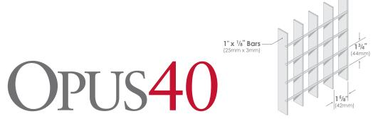
The extremely rigid characteristics of the popular Opus40 design provide a closely spaced nominal square pattern with increased strength and security. This product is ideally suited for shorter fences and infill panel requirements.
