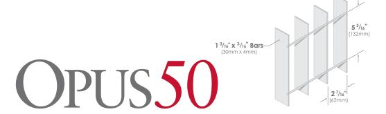
Designed to provide increased depth and strength of the main elements, Opus50 incorporates a deeper bar section while maintaining the same timeless spacing pattern of the most popular Opus10 design.
